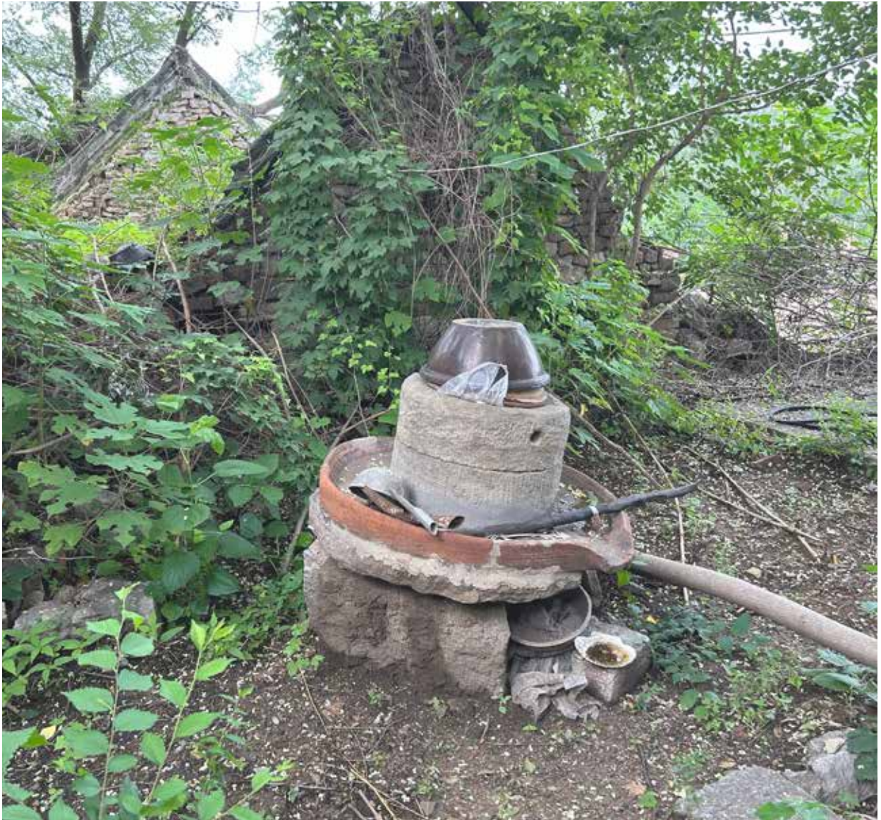
Figure 34. Stone mill in the courtyard of an abandoned old house. The stone mill is used for grinding grains such as wheat, rice, or corn. In the past, this mill would have been a crucial part of daily life. The grain is fed into the centre, and as the stones rotate, it crushes the grain into flour or meal.
