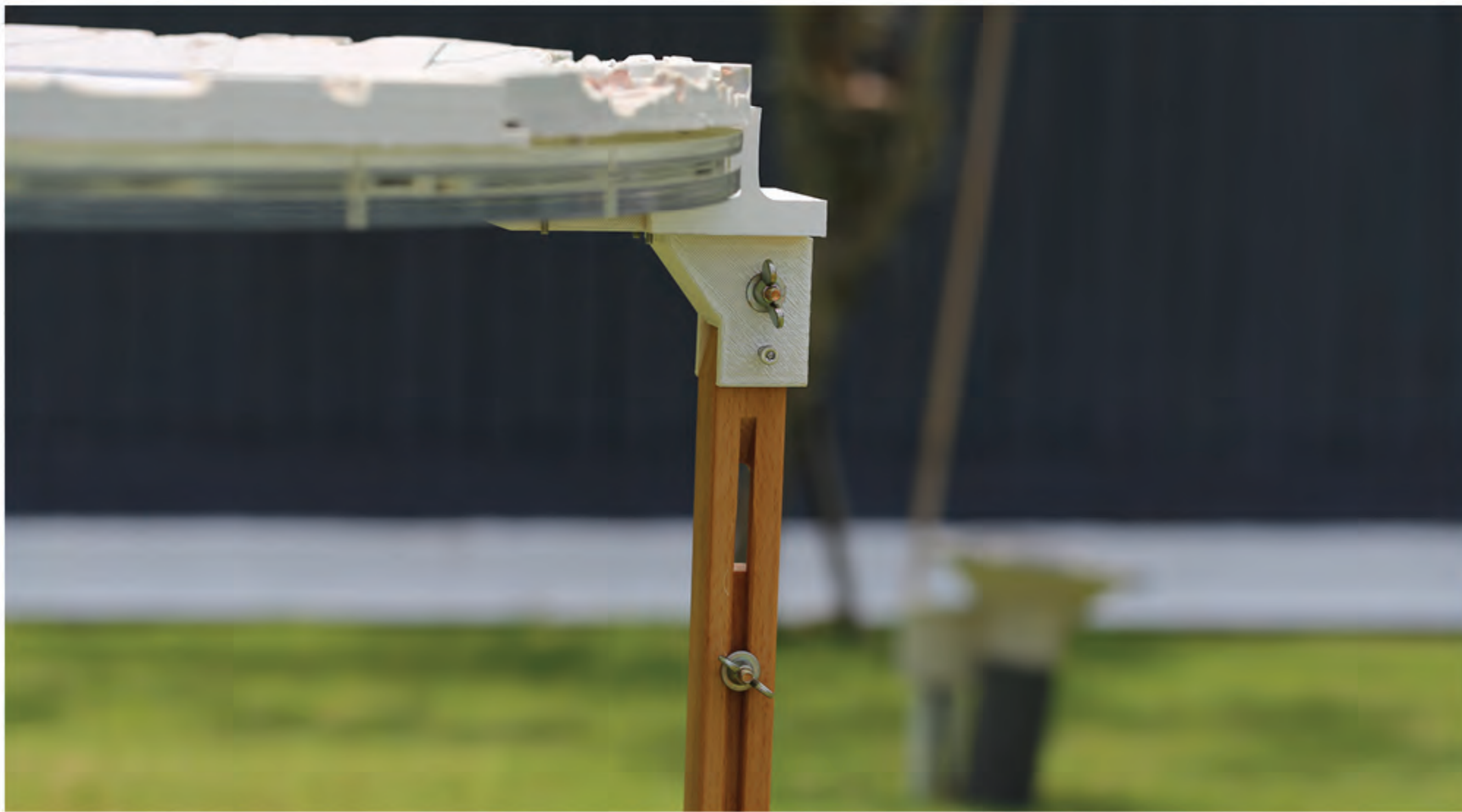
photograph of the leg, and connection via the 3D-printed leg bracket.
