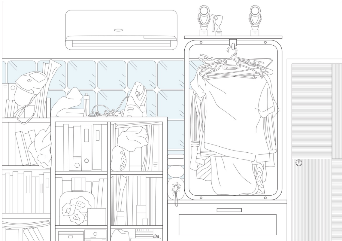
Figure 2.24 Clutter obscuring view through glass brick wall
