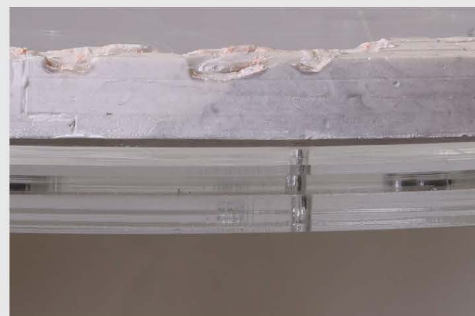
3 pieces of acrylic were used to reinforce the surface of the map.
