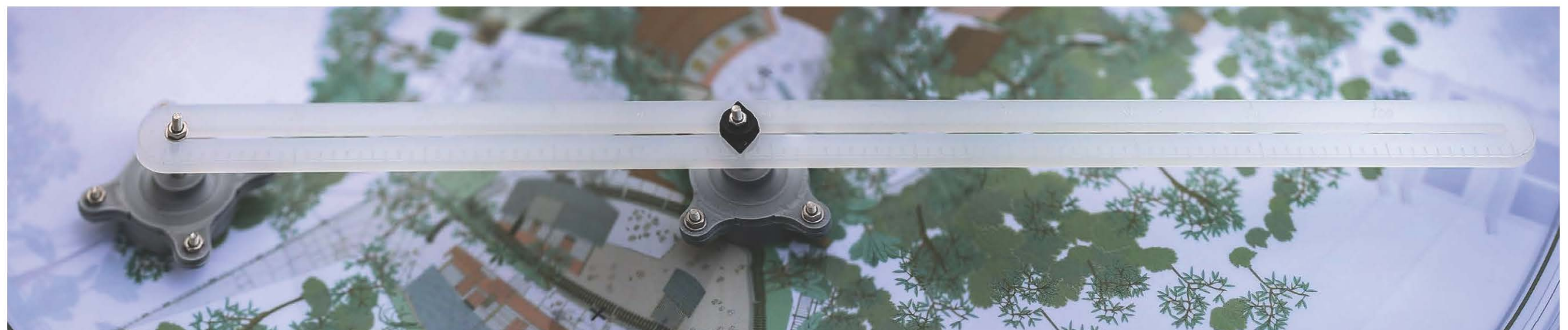
magnets within the acrylic panels would anchor the ruler on uneven topography
